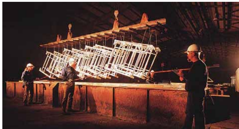
Australia Post pallet bases being galvanised.
